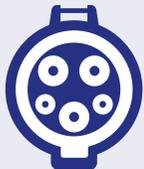
If you're using a **Tethered Type 1 connector**, make sure you insert the connector firmly. DO NOT press the button while connecting the cable to the vehicle. The button should only be used to release the cable.
