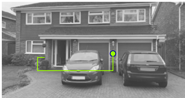
Proposed cable route – where you would imagine the cables to run from your main electricity supply into the charging unit (internal and external of the property)
